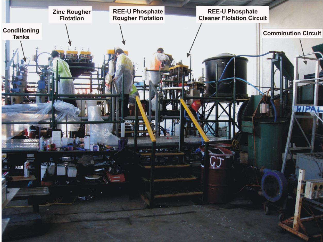
Figure 1. Kvanefjeld flotation circuit – stage one pilot plant, SGS Oretest, Perth. The plant was run continuously for 15 hours to produce a zinc (sphalerite) concentrate, and a REE-U phosphate mineral concentrate. The ability to effectively concentrate the REE-U bearing phosphate minerals into a small mass fraction represents a critically important breakthrough in establishing the optimal process flow-sheet for the Kvanefjeld project.
