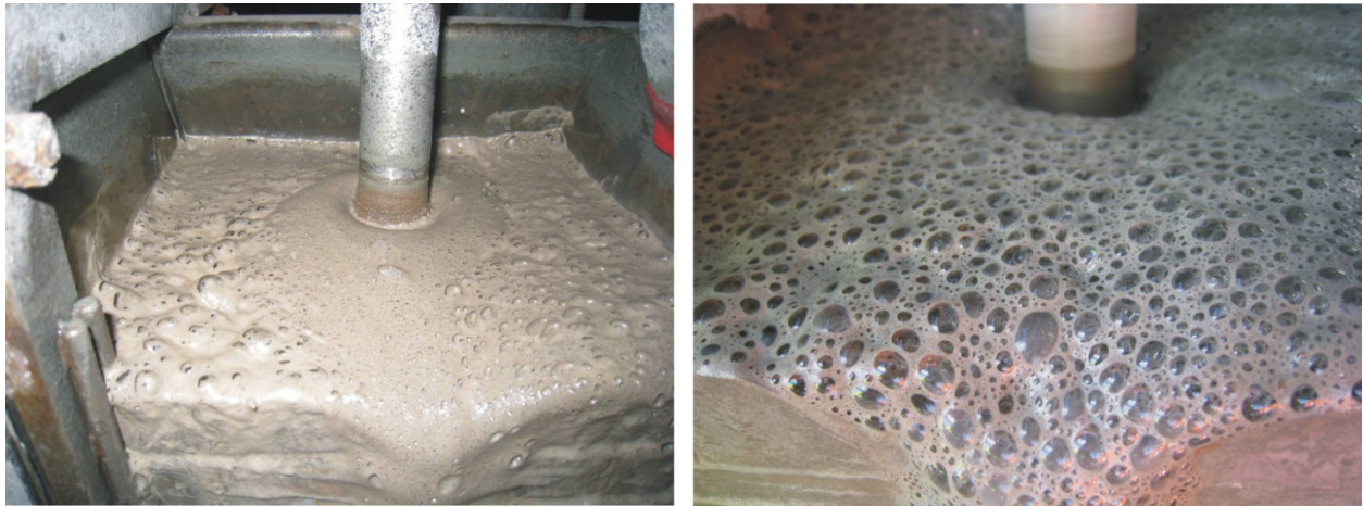
Figure 2. The REE-phosphate cleaner cell (left), and a close-up of the REE-phosphate mineral froth.
